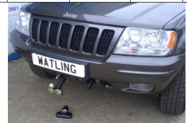
Jeep Grand Cherokee Mk2 with additional centre receiver
